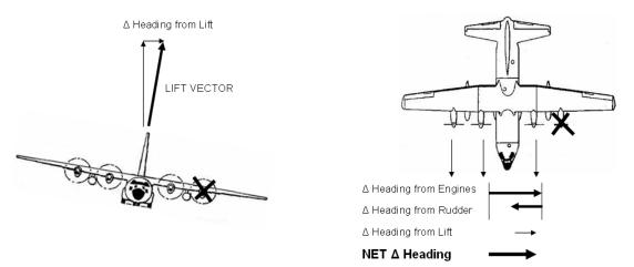
Lastly, look at an extreme scenario (below). The aircraft is in 60 degrees of bank into the dead engine. The result is a large turn in the direction the aircraft is banking.
