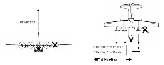
Next, let's look at the 5 degree adverse bank picture (below). The lift vector now generates a heading change in the wrong direction and induces a larger turn. Again, according to the Dash-1-1, the pilot would have to accelerate 37 knots to generate enough rudder force to counteract this turn.
